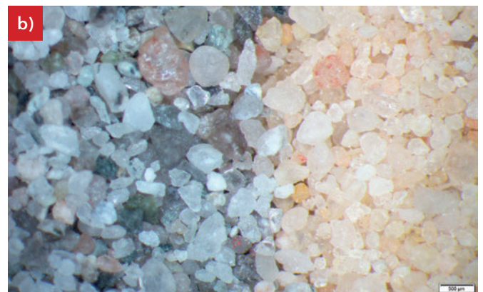
Fig. 6: a) KWS - Desert sand, b) Washer sand 0/1 - desert sand. (Microscopic images with 18x magnification)
